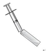
To stop bubbles forming, let the sample flow down the inside.
